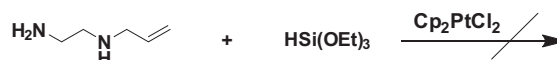
Scheme 2. (Dicyclopentadiene) platinum(II) dichloride catalyst for the hydrosilylation of the diamino chelating alkene with triethoxysilane.
